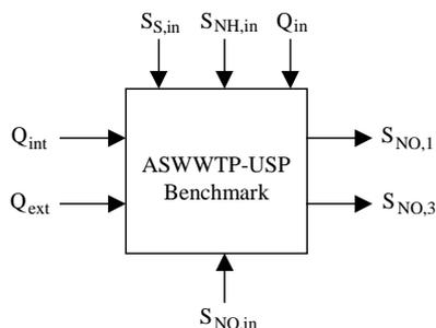
Fig. 2. Signals for subspace identification.
