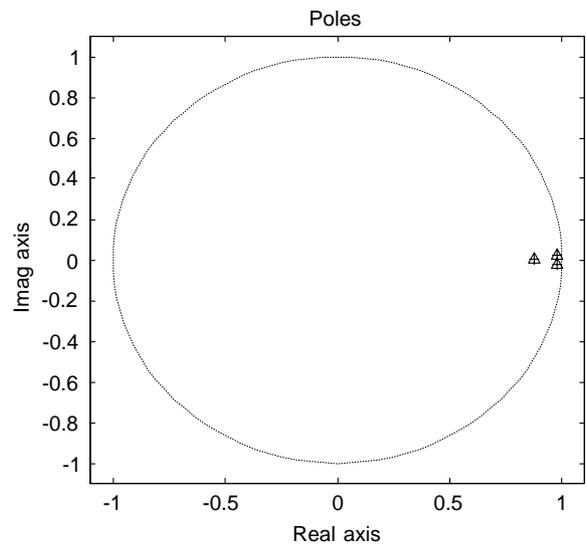
Fig. 9. Location of the poles of the DSR-models.
