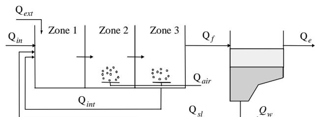
Fig. 1. Layout of the ASWWTP-USP benchmark.
