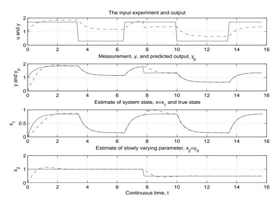
Figure 1: Simulation of the system in Example 7.1 with the state estimator in parallel. Butterworth observer polynomial with gain as in Equation (77).
