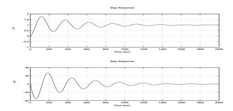
Figure 1: Example of an oscillating feedback system with initial wrong tuning. Feedback control of integrating plus time delay process,  $h_p(s) = \frac{e^{-s}}{s}$ , and PIcontroller  $h_c(s) = K_p \frac{1+T_i s}{T_i s}$  with initial settings as in (6).
